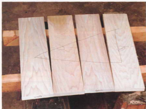
Panel boards are matched for appearance. A large triangle records the order and placement. When gluing up multiple panels, use different marks to distinguish them.
