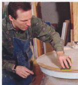
Place the workpiece on a piece of rigid foam. Dampen the veneer along the edge and slide the assembly into the vacuum bag.
