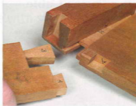
Place letters, numbers and Roman numerals in inconspicuous places to designate mating joints. Here, a table leg is matched with a drawer rail and apron.
