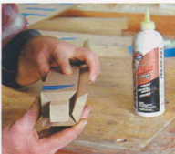
Wrap up the leg. Spread glue on all of the interior surfaces, including the core. Then wrap the four mitered sections around the core and secure the assembly with additional tape.
