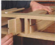
Glides span the dividers. Center dividers are sandwiched between two filler boards that house the drawer glides.
