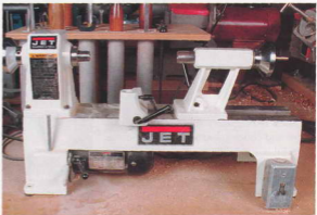
Entry-level lathe. Small but well-proportioned, a midi-lathe offers an economical way to begin turning on a solid machine.
