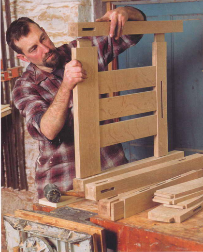
Assemble the ends. First fit the slats to the apron and lower rail, then set the assembly into the mortises on the legs.
