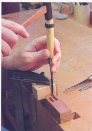
Help with the handwork. A thick block of wood clamped firmly to the workpiece serves as a guide to chisel the ends of the mortises true and square.
