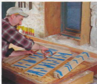
Strips of masking tape act as clamps. Set the mitered edges of the legs tightly against each other, then tape them together.
