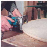
Once the glue has cured, clean up the edge. A router or laminate trimmer equipped with a flush-trimming bit will do the job.
