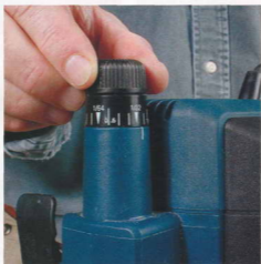
Fine-tune the depth of cut by turning a knob or dial. The Bosch, DeWalt and Festool allow micro-adjustments immediately after the housing has been plunged.
